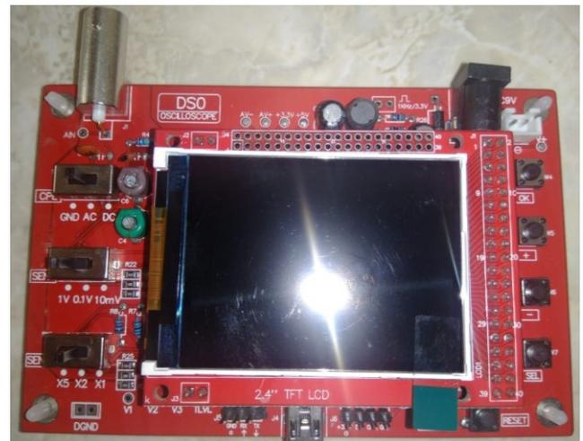
Fig. 11. DSO138 Digital Oscilloscope
