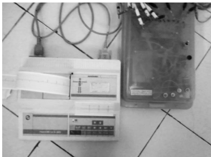
Fig 8. Testing Human Cardiac Simulator Using ECG Recorder
