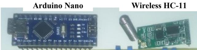
Fig. 14. Digital part of Central Monitor
