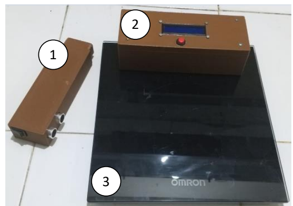
FIGURE 3. Digital anthropometry for stunting detection. Notes: one (1) is a tool to measure the body height wirelessly, two (2) is a control box which consist of Microcontroller ESP32, and three (3) indicate.
