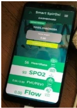
FIGURE 5. Final Design of Android Application Spirometry with Oximeter IoT
