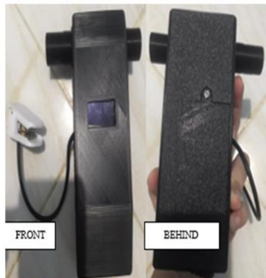
FIGURE 4. Final Design of Module Spirometry with Oximeter IoT
