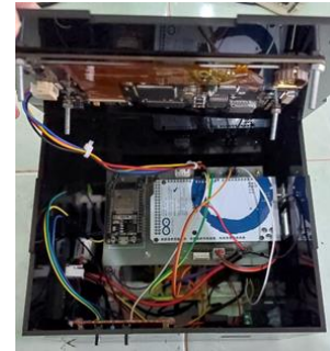
FIGURE 6. The design of circuit to process the measurement NIBP and Weight
