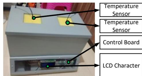
**FIGURE 3.** Digital Thermometer Calibrator Device Design
