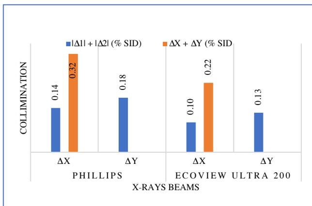
FIGURE 7. Results of the collimation field difference test with X-Ray Beams.
