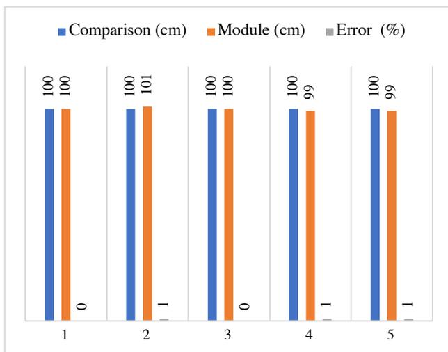
FIGURE 4. Chart contains of distance measurement results which include the data module, comparison and error value.
