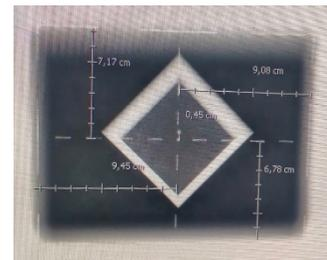
FIGURE 9. Collimation test results on the ecoview ultra 200 x-ray machine, the value of the light lap for x1 is 7 cm, x2 is 7 cm, y1 is 9 cm, and y2 is 9 cm. Then the x-ray values are obtained for x1 6.7 cm, x2 values are 7.1 cm, y1 values 9.4 cm, and y2 values 9.08 cm.
