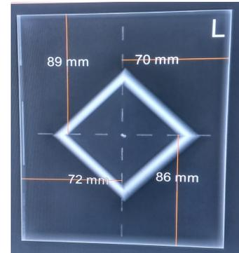
FIGURE 8. Results of the collimation test on a phillips x-ray machine, the value of the light lap for x1 is 7 cm, x2 is 7 cm, y1 is 9 cm, and y2 is 9 cm. Then for the value of the x-ray lap, x1 is obtained 7cm, for x2 7.2 cm, for y1 8.6 cm, for y2 8.9 cm.
