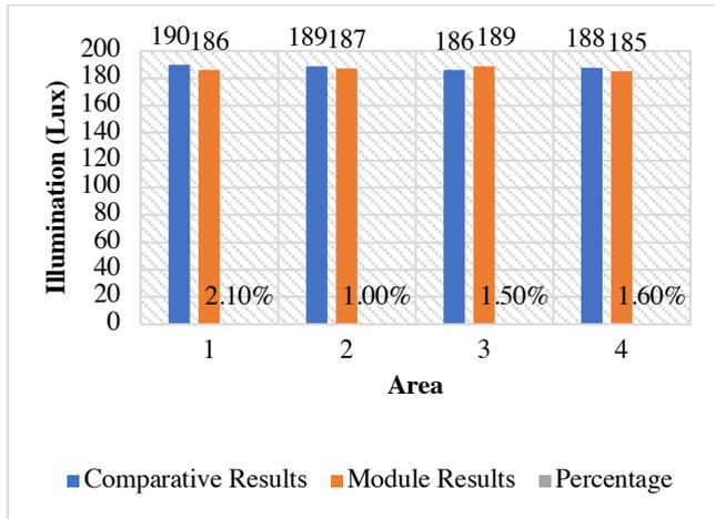
FIGURE 3. Chart contains of the Illumination measurement result Measurements were made by comparing the module with the Digital Light Meter Model 5202 KYORITSU ELECTRICAL INSTRUMENTS WORKS, LTD.
