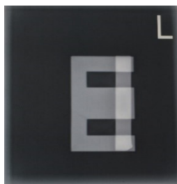
FIGURE 16. Digital Radiography (DR) Image Results at the Setting of 70 kV 40 mA 200 ms had a good image.
