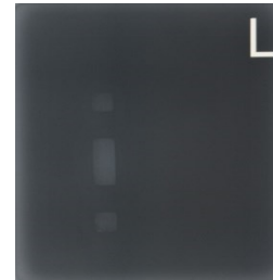
FIGURE 17. Digital Radiography (DR) Image Results at the Setting of 70 kV 40 mA 1 second resulted in the image that was not visible because it took too long to receive a dose, leading to too much data read.
