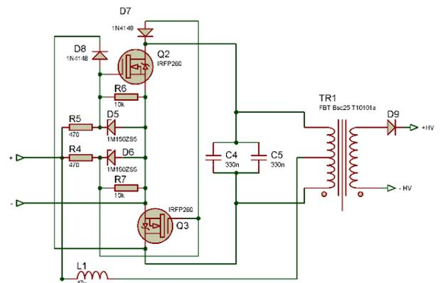
FIGURE 4. Mazzili ZVS Flyback Converter
