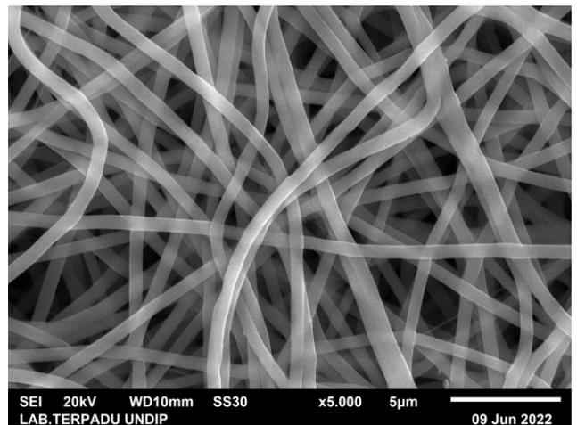
FIGURE 11. Nanofiber captured under scanning electron microscopy
