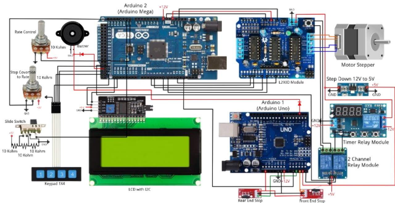
FIGURE 1. Schematic Design of The Syringe Pump
