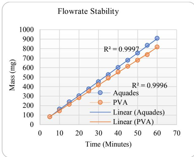
FIGURE 12. Linearity flowrate indicates that flowrate is stable
