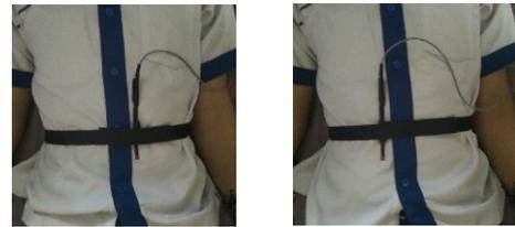
Fig. 10. Sensor placement to measured the respiration (a) left (b) right side
