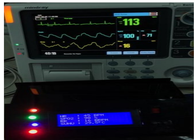
Fig. 3. The Display of Module Measurement Results with Comparison of respiratory rate values
