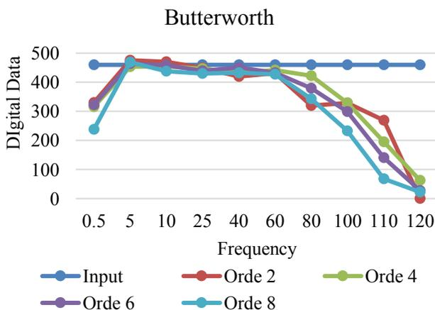
Fig 7. Digital Filter using Butterworth Type
