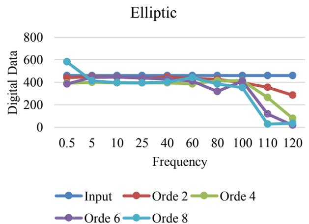
Fig 10. Digital Filter using Elliptic Type
