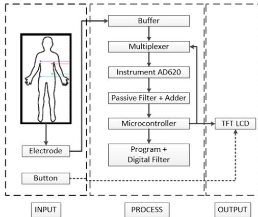
Fig 1. The diagram block of development of a low-cost and efficient ecg devices with II digital filter design.
