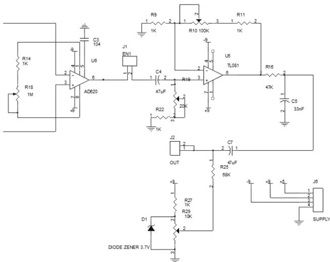
Fig 5. Circuit of Instrumentation
