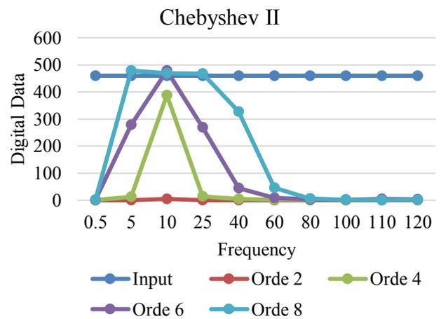
Fig 9. Digital Filter using Chebyshev II Type
