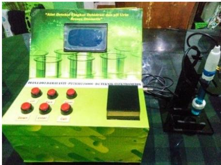
Fig. 12. Automatic Dehydration and pH Urine Level Detection Device
