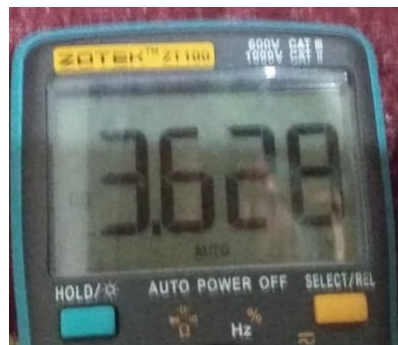
Fig. 7. MPXV7002DP Sensor output result after the patient breathes
