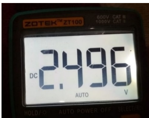
Fig. 6. MPXV7002DP Sensor output result before the patient breathes
