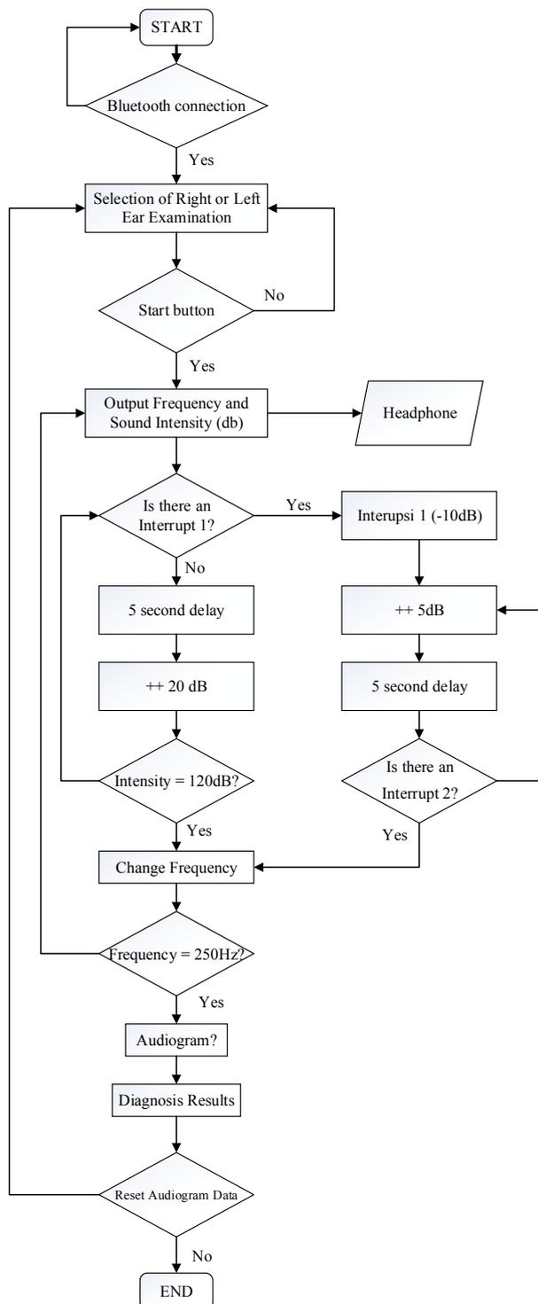
Fig. 2. The Flowchart of Automatic Pure Tone Audiometer
