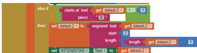
Fig. 15. The Mit App Inventor 2 Program when receiving B record is initialized as a intensity data
