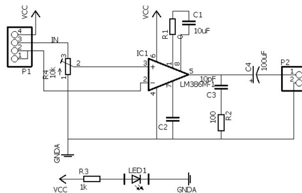
Fig. 6. Amplifier LM386 with gain 200
