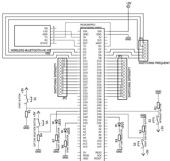
Fig. 10. Mikrokontroler Arduino ATmega2560 Pro Mini circuit
