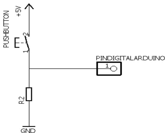
Fig. 9. Pull-up Resistor
