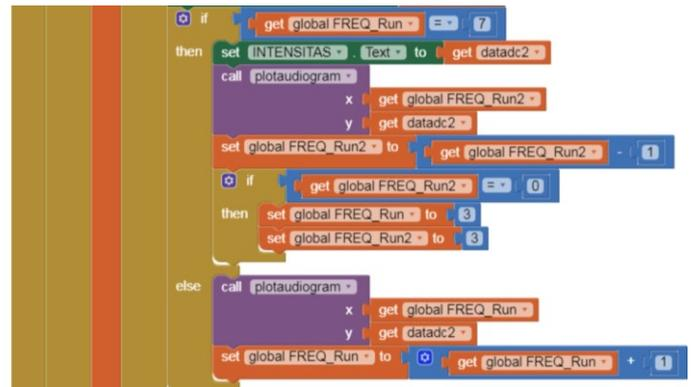
Fig. 16. The Mit App Inventor 2 Program when performing data plotting
