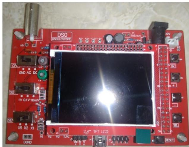
Fig. 11. DSO138 Digital Oscilloscope
