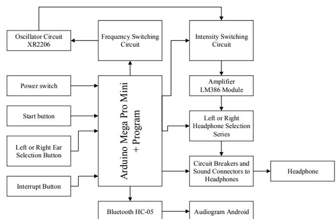
Fig. 1. A block diagram of Automatic Pure Tone Audiometer
