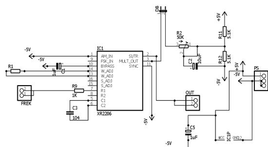
Fig. 4. Generator Frekuensi 250-8000Hz with XR2206
