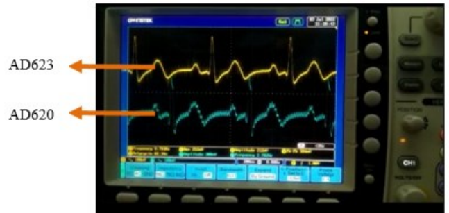
FIGURE 8. The results of the ECG signal obtained from the instrumentation amplifier of bipolar supply and Single supply.
