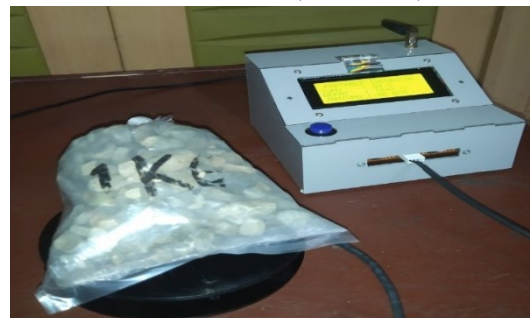
FIGURE 8. Testing weight measuring circuit of portable incubator monitoring tool with short message service (SMS) notifications.
