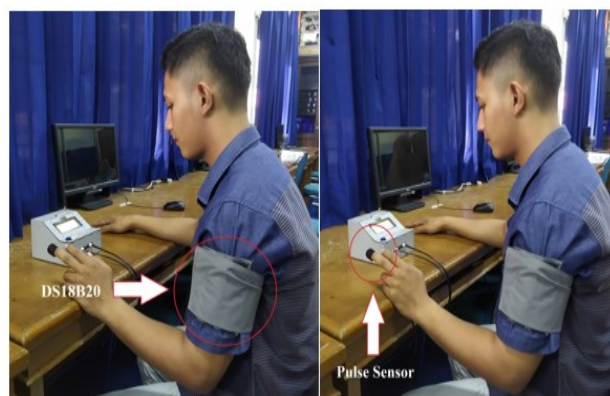
FIGURE 7. Testing heart rate and body temperature circuits of portable incubator monitoring tool with short message service (SMS) notifications
